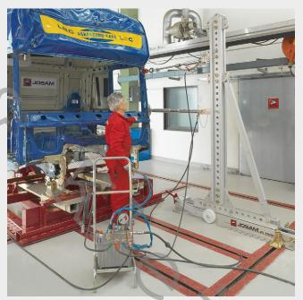
The JOSAM cab bench works together with our aluminium straightening towers and extra accessories related to pulling and pressing.
