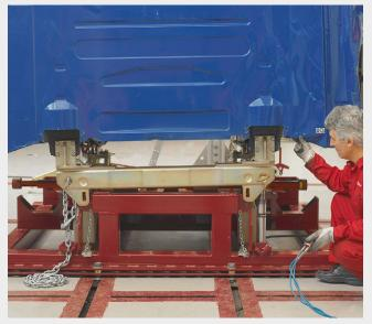
In addition, the rear part of the cab bench is moveable, which enables vertical straightening of a distorted cab. The cab is pressed upwards to its correct position so that it is in the same vertical line as the cab bench itself.
