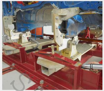
The four mounting points of the damaged cab are anchored to the bench by means of specially designed adapter sets for each cab model. Badly displaced front mounting points are held and pressed into the correct position by using a hydraulic cylinder and moveable jig members.
